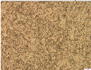
Fig. 5 AISI H21 structure after 100 cycles, nital etch, equiaxed grains and large carbides
