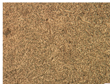
Fig. 4 AISI H21 structure after 80 cycles, nital etch, lower bainite and coalesced carbides
