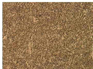
Fig. 2 AISI H21 initial structure, nital etch, martensite with fine carbides
